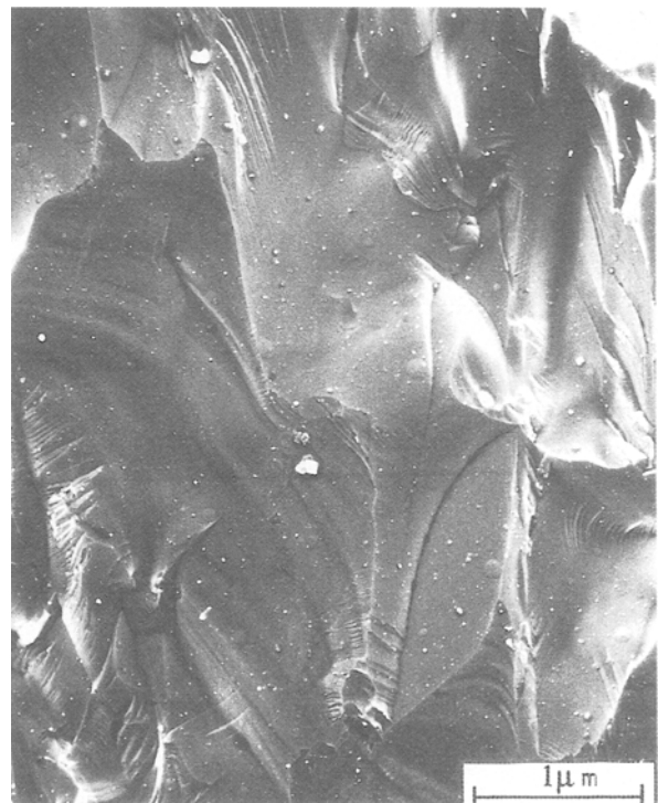
Figure 2 Fracture surface of CVD \text{Si}_3\text{N}_4 four-point bend test showing transgranular failure.
